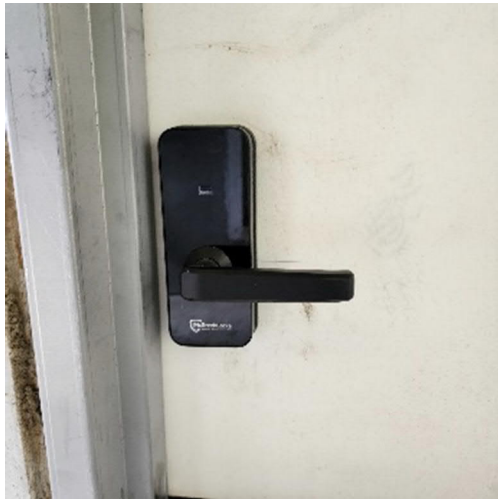
Figure 1 Unexposed side view of the tested hardware
