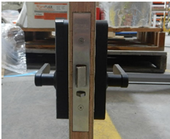
Figure 3 Latch edge side view of the tested hardware
