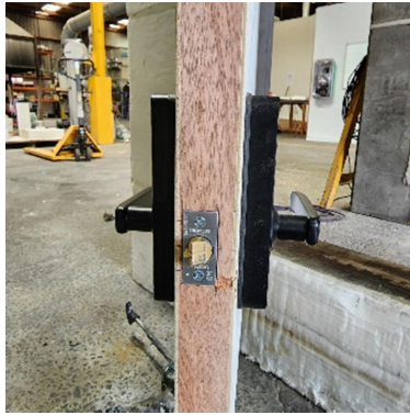
Figure 3 Latch edge view of the tested hardware
