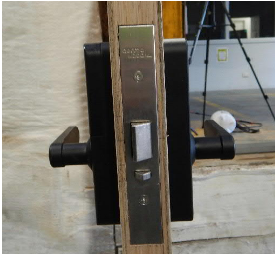
Figure 3 Latch edge view of the tested hardware
