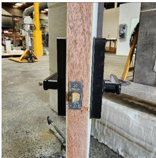
Figure 3 Latch edge side view of the tested hardware
